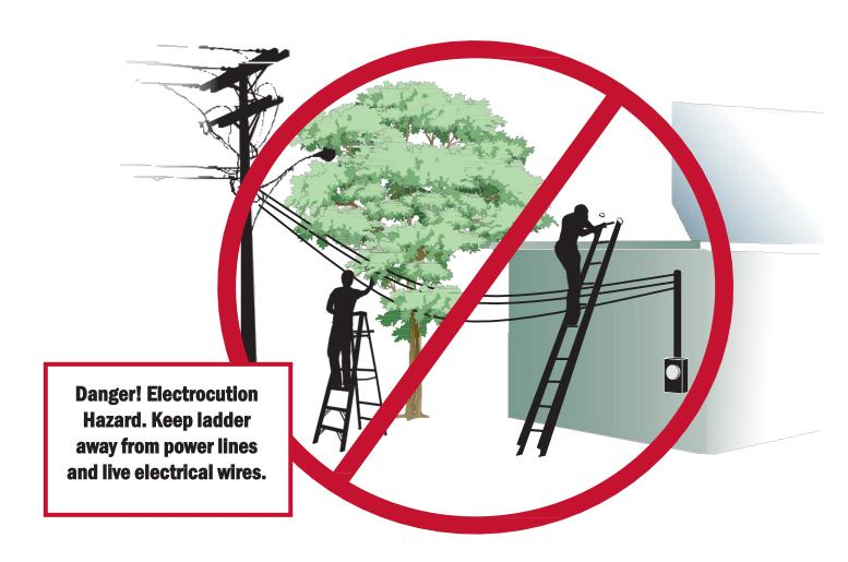
Despite these and other warnings, electrocutions still occur each year. To avoid this hazard, CPSC advises you to use a ladder that does not conduct electricity, such as fiberglass with non-conductive side rails when working near overhead wires. Non-conductive ladders should be kept clean to maintain their non-conductive safety properties.
